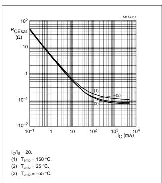
Fig.10 Equivalent on-resistance as a function of collector current; typical values.
